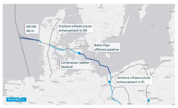
Figure 1 Overview of the five components of Baltic Pipe. Route and compressor station location are indicative, and not specific.
